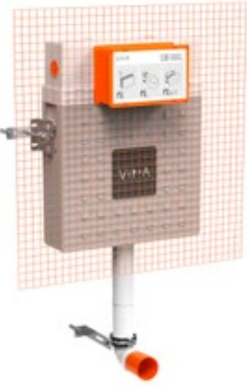
Concealed cistern 12cm, regular for back-to-wall WCs, 3/6 litre H: 730-830mm W: 420mm P: 120mm
