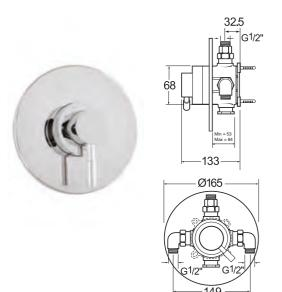
VALVE: INLET CONNECTIONS: Thermostatic 15mm Compression OPERATION: WORKING PRESSURE: 0.1 - 5.0 bar Single control for flow and temperature
