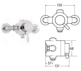
VALVE: Thermostatic INLET CONNECTIONS: 15mm Compression WORKING PRESSURE:
