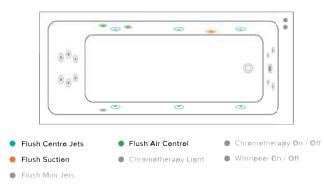
6 Side Jets, Pneumatic Control, Flush Air Control, Flush Suction
