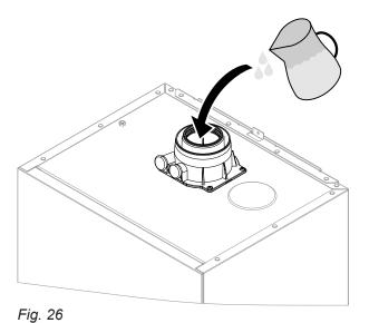
Pour at least 0.3 I of water into the flue gas connection.
