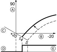
Fig. 64 Example 2: Adjusting the reduced set room temperature from 5 °C to 14 °C
