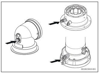
Fig. 102 Flue gas test port
