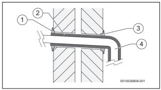
Fig. 41 Through the wall lagging example
