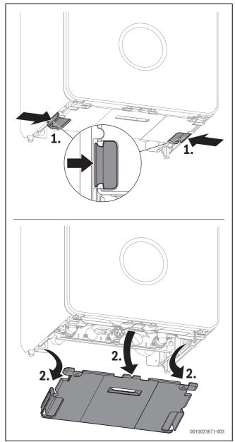
*Fig. 77 Removing bottom panel*
