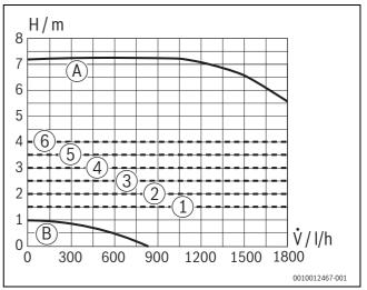
Fig. 113 Pump characteristic maps and pump curves
