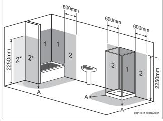
Fig. 13 Bathroom installations
