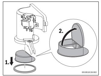
Fig. 85 Non-return valve in the air-gas manifold
