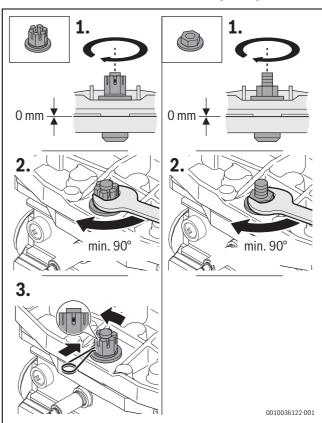
Fig. 83 Tightening the screws
