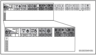
Fig. 61 Power supply (power cables) terminal strip
