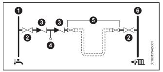
Fig. 11 External filling loop system fill example
