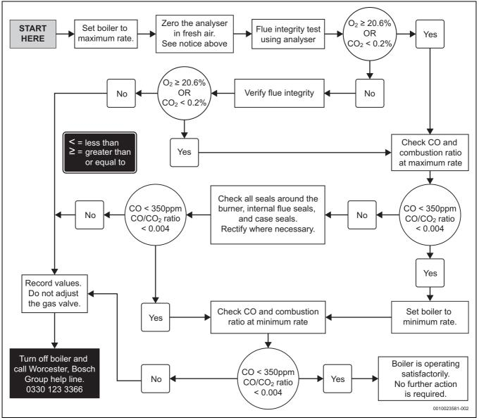
Fig. 73 Commissioning checks flow chart
