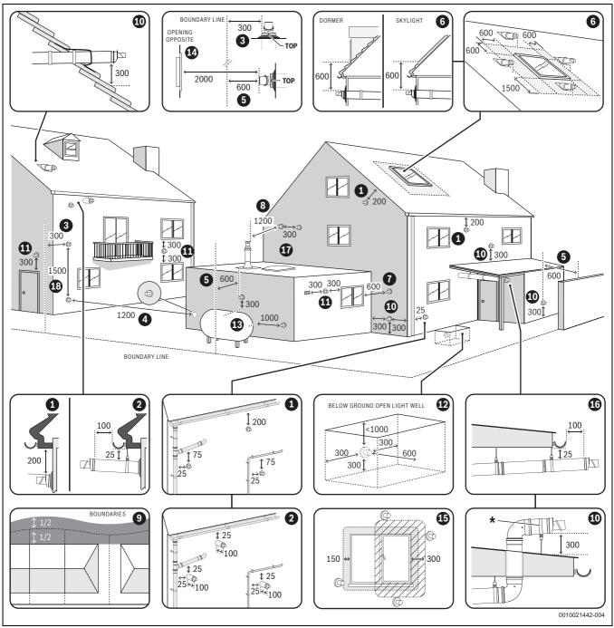
Fig. 32 Horizontal flue terminal positions
