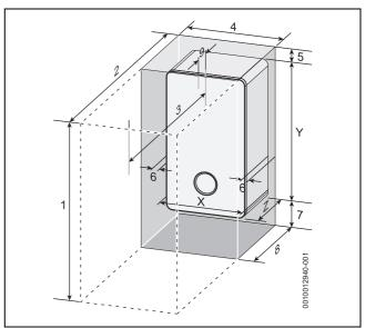
Fig. 14 Appliance minimum clearances
