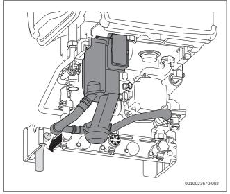
Fig. 54 Condensate connection
