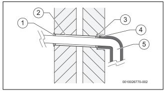
Fig. 37 Additional protection for transition through a wall
