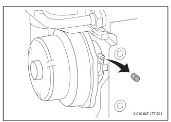
Fig. 79 Fan pressure test point
