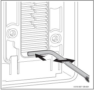
Fig. 92 Cleaning debris
