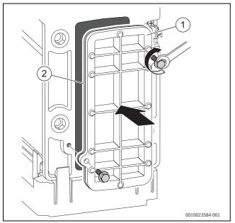
Fig. 93 Re-fitting the access cover
