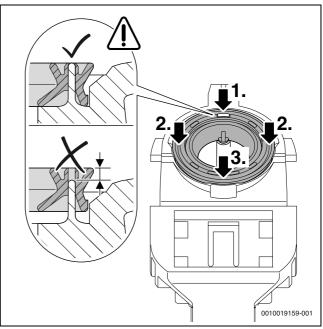
*Fig.* 98 *Pressing on the gasket*
