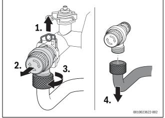
Fig. 106 Removing pressure relief valve
