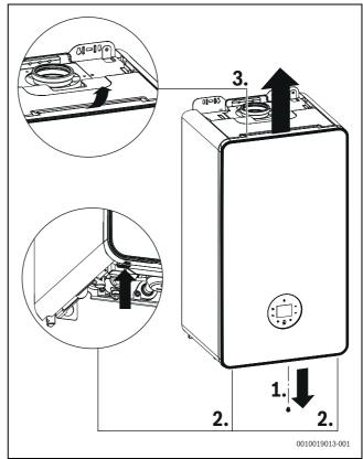
Fig. 78 Removing outer case
