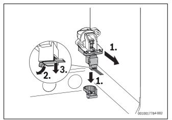
Fig. 110 Removing the motor of the 3-way valve
