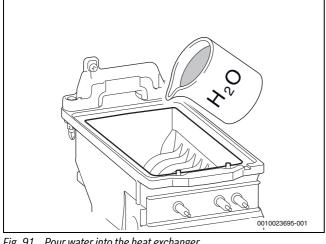
Fig. 91 Pour water into the heat exchanger
