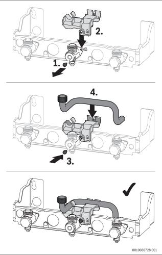
Fig. 49 Connect PRV discharge pipe
