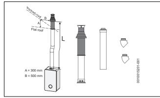
Fig. 28 Vertical flue option
