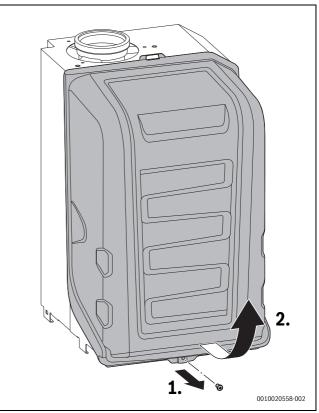
Fig. 100 Removing the combustion cover
