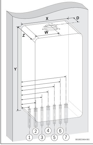
Fig. 2 Pipe and flue outlet dimensions
