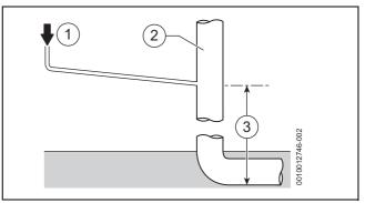
Fig. 34 Disposal to soil vent stack
