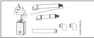
Fig. 22 Horizontal flue option
