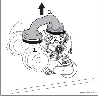
Fig. 107 Removing the gas pipe
