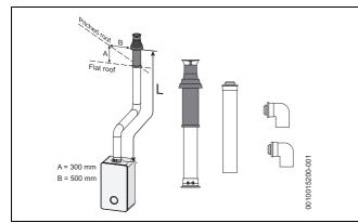
Fig. 27 Vertical flue option
