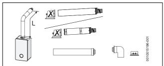
Fig. 23 Horizontal flue option
