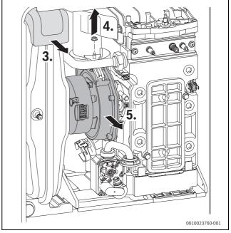
Fig. 87 Fan removal
