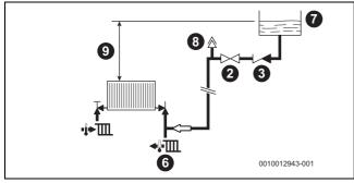
Fig. 12 Top-up tank system fill example
