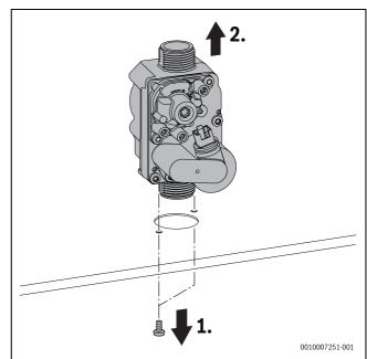
Fig. 109 Removing the gas control valve
