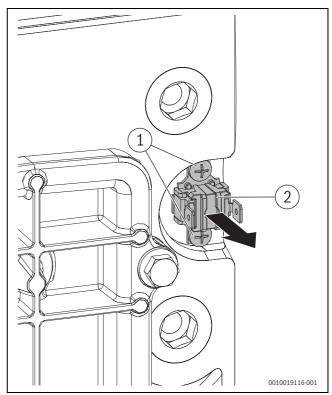
Fig. 104 Removing overheat thermostat
