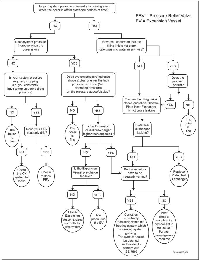
Fig. 112 System gassing flow chart
