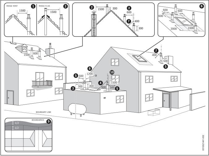
Fig. 31 Vertical flue terminal positions
