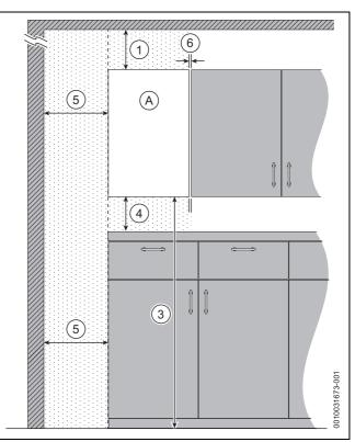
Fig. 16 Reduced front maintenance clearances - Front view
