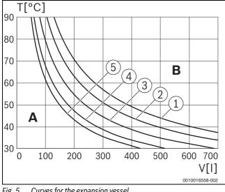
Fig. 5 Curves for the expansion vessel
