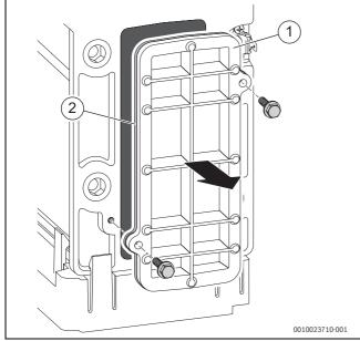
Fig. 88 Access cover removal
