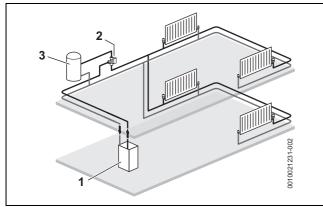
Fig. 8 3-way valve, cylinder and heating zone
