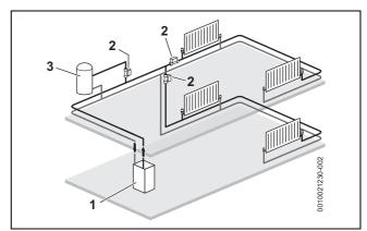
Fig. 7 Cylinder and 2 x heating zones
