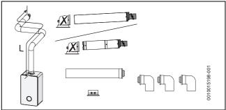
Fig. 25 Horizontal flue option
