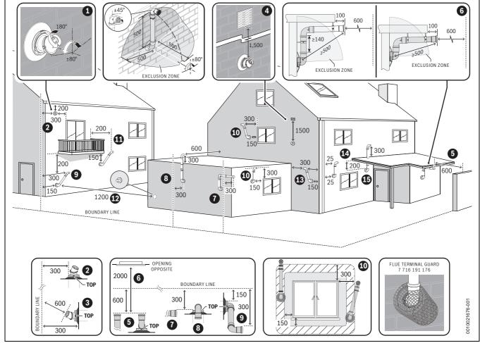
Fig. 33 Plume re-direct and plume management terminal positions
