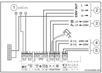
Fig. 65 External controls connections example
