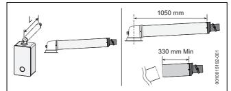
Fig. 19 Horizontal flue option
