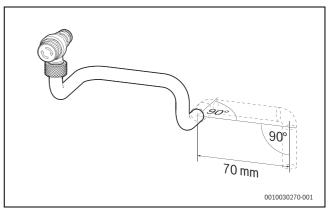
Fig. 52 Discharge pipe to existing CDI classic position (not in the hardware pack)
