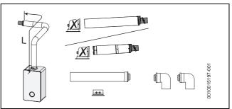
Fig. 24 Horizontal flue option
