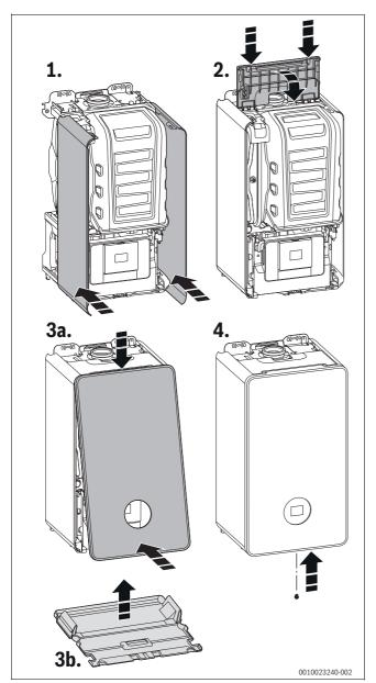
Fig. 76 Fitting the appliance casing
