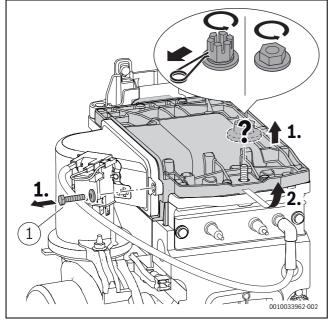
Fig. 81 Removing the burner cover
