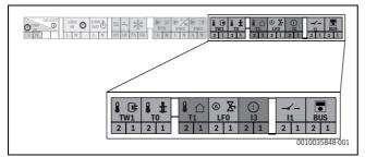
Fig. 62 Low voltage (signal cables) terminal strip
