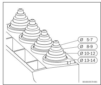
Fig. 60 Adapting the strain relief to the cable diameter
