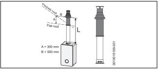
Fig. 26 Vertical flue option
