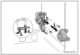
Fig. 111 Removing the 3-way valve
