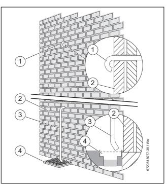
Fig. 42 Pressure relief pipework
