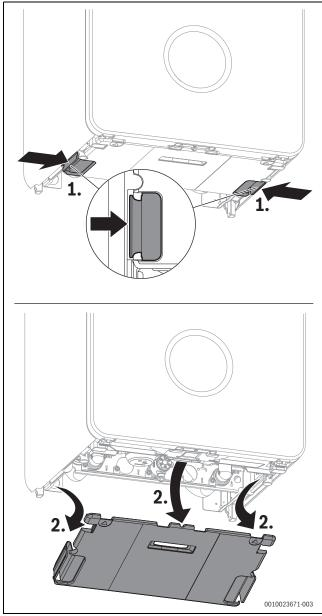
Fig. 77 Removing bottom panel
