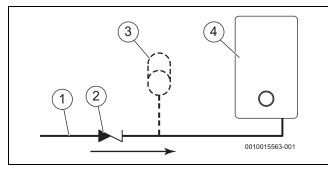
Fig. 9 Mini expansion vessel location
