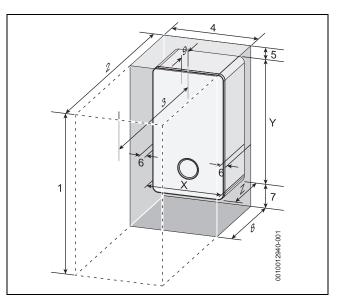
*Fig. 11 Appliance minimum clearances*
