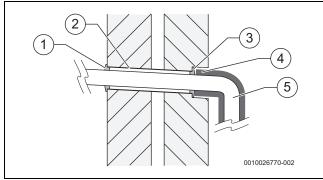
Fig. 34 Additional protection for transition through a wall
