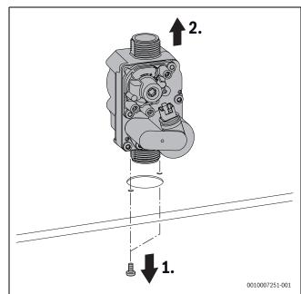
Fig. 109 Removing the gas control valve
