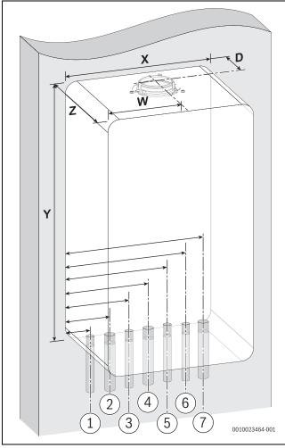
*Fig. 2 Pipe and flue outlet dimensions*
