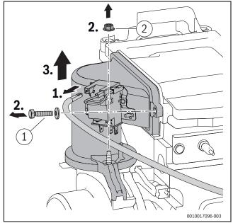
Fig. 84 Removing the air-gas manifold
