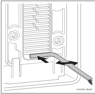
Fig. 92 Cleaning debris
