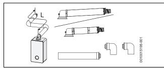
Fig. 19 Horizontal flue option
