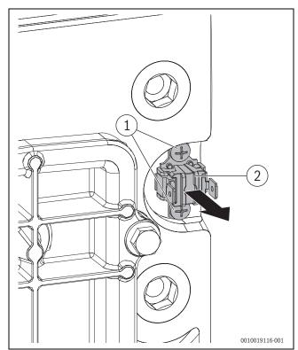
Fig. 104 Removing overheat thermostat
