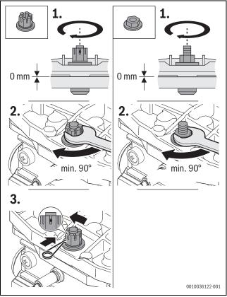
Fig. 83 Tightening the screws
