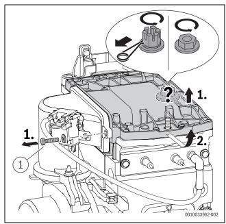
Fig. 81 Removing the burner cover
