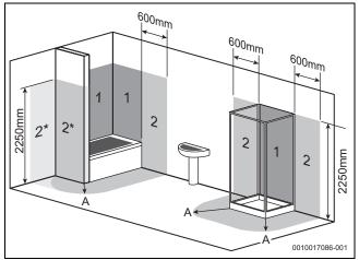
Fig. 10 Bathroom installations
