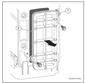
Fig. 88 Access cover removal
