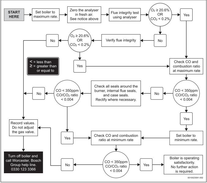
Fig. 73 Commissioning checks flow chart
