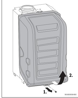
Fig. 100 Removing the combustion cover
