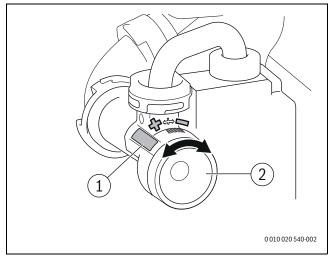
Fig. 101 Setting the adjustable venturi
