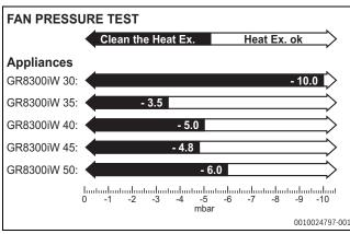
Fig. 80 Fan pressure test values
