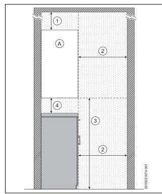
Fig. 12 Reduced front maintenance clearances - Side view
