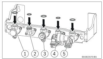
Fig. 45 Fitting the sealing washers
