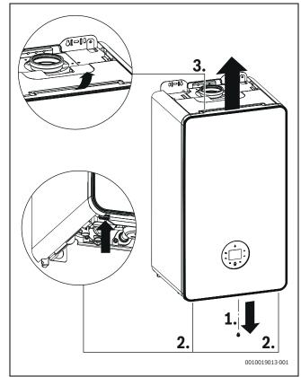
Fig. 78 Removing outer case
