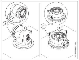
Fig. 55 Flue turret/adaptor connection
