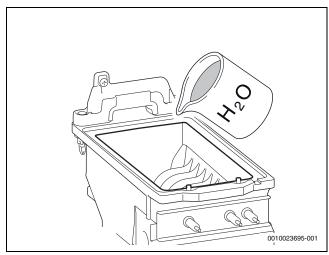
Fig. 91 Pour water into the heat exchanger
