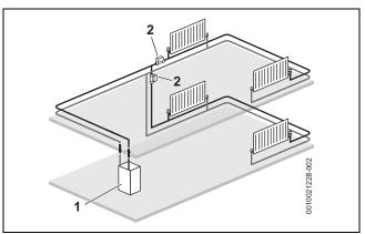
Fig. 7 Separated heating zones
