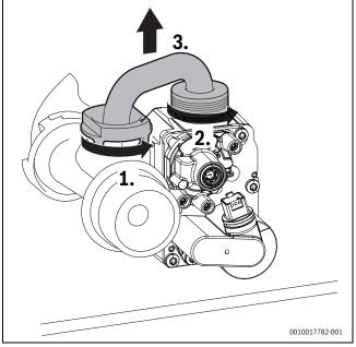
Fig. 107 Removing the gas pipe
