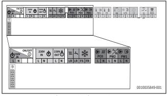
Fig. 58 Power supply (power cables) terminal strip
