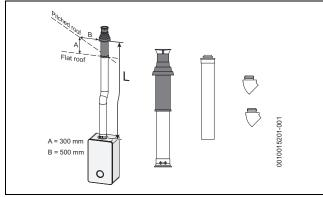
Fig. 25 Vertical flue option
