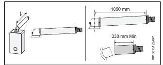
Fig. 16 Horizontal flue option
