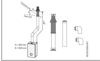
Fig. 24 Vertical flue option
