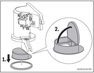
Fig. 85 Non-return valve in the air-gas manifold
