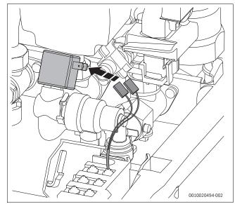
Fig. 60 Connecting the automatic filling facility
