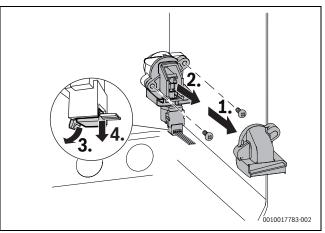
Fig. 113 Removing the 3-way valve
