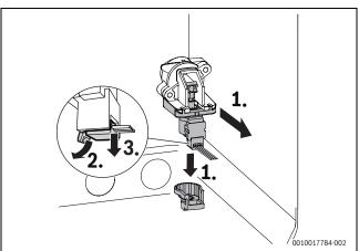
Fig. 112 Removing the motor of the 3-way valve
