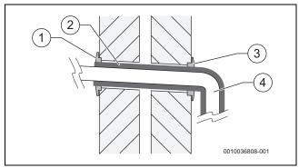
Fig. 38 Through the wall lagging example
