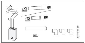
Fig. 22 Horizontal flue option
