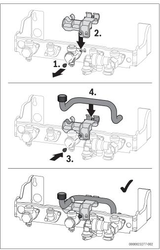
Fig. 46 Connect PRV discharge pipe
