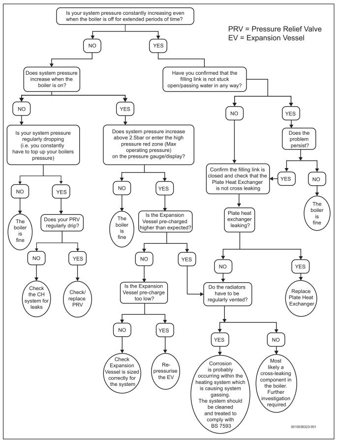
Fig. 115 System gassing flow chart
