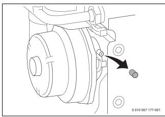
Fig. 79 Fan pressure test point
