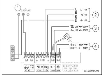
*Fig. 63 External controls connections example*
