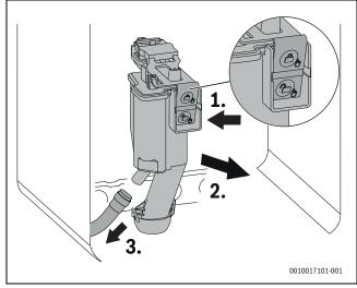
Fig. 96 Removing the condensate trap
