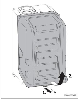
Fig. 68 Removing the combustion cover
