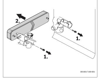
Fig. 114 Removing the plate heat exchanger
