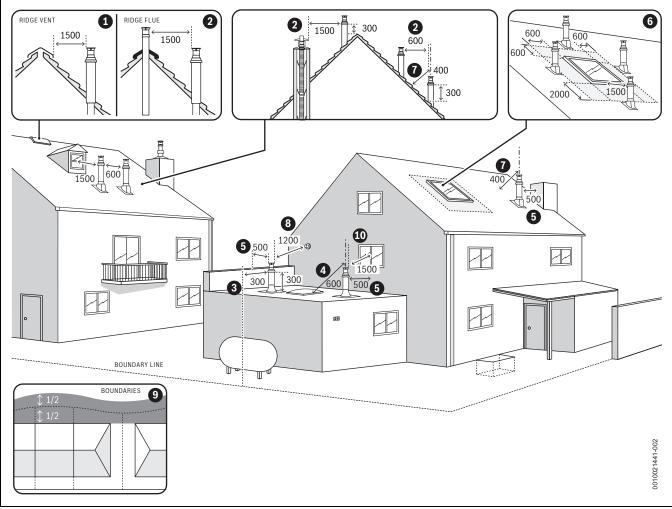
Fig. 28 Vertical flue terminal positions
