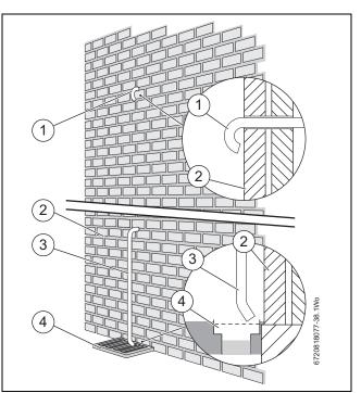
Fig. 39 Pressure relief pipework
