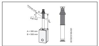
Fig. 23 Vertical flue option
