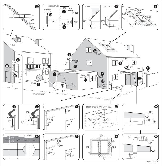
Fig. 29 Horizontal flue terminal positions
