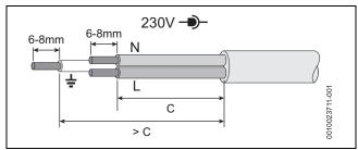
Fig. 61 Power supply (power cables) preparation
