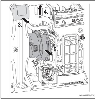
Fig. 87 Fan removal
