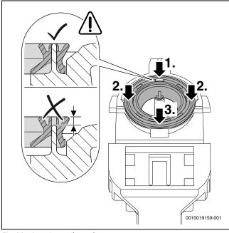
Fig. 98 Pressing on the gasket
