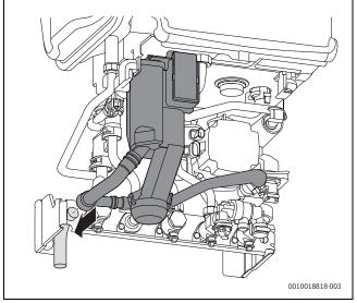
Fig. 51 Condensate connection
