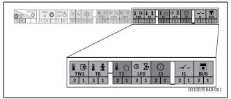
Fig. 59 Low voltage (signal cables) terminal strip
