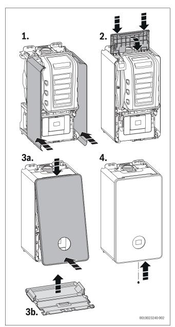
Fig. 76 Fitting the appliance casing
