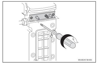
Fig. 94 Installing electrode set
