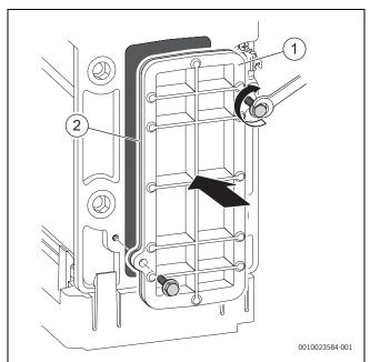
Fig. 93 Re-fitting the access cover
