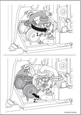
Fig. 86 Venturi removal
