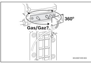
Fig. 95 Checking for leaks with an inspection mirror. Observe for misting.
