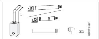
Fig. 20 Horizontal flue option
