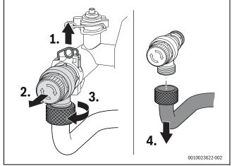
Fig. 106 Removing pressure relief valve
