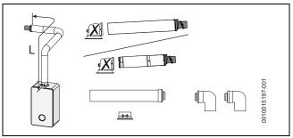
Fig. 21 Horizontal flue option
