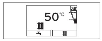
The basic display shows the current condition of the product. If you press a selection button, the activated function is displayed in the display.
