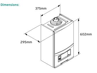
Note: A minimum of 600mm clearance in front of the boiler is required to enable easy access for servicing. This may be provided by an accessible door.
