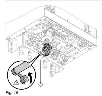
When carrying out any work on gas connection fittings, hold with a suitable tool. Never transfer any forces to the internal components.
