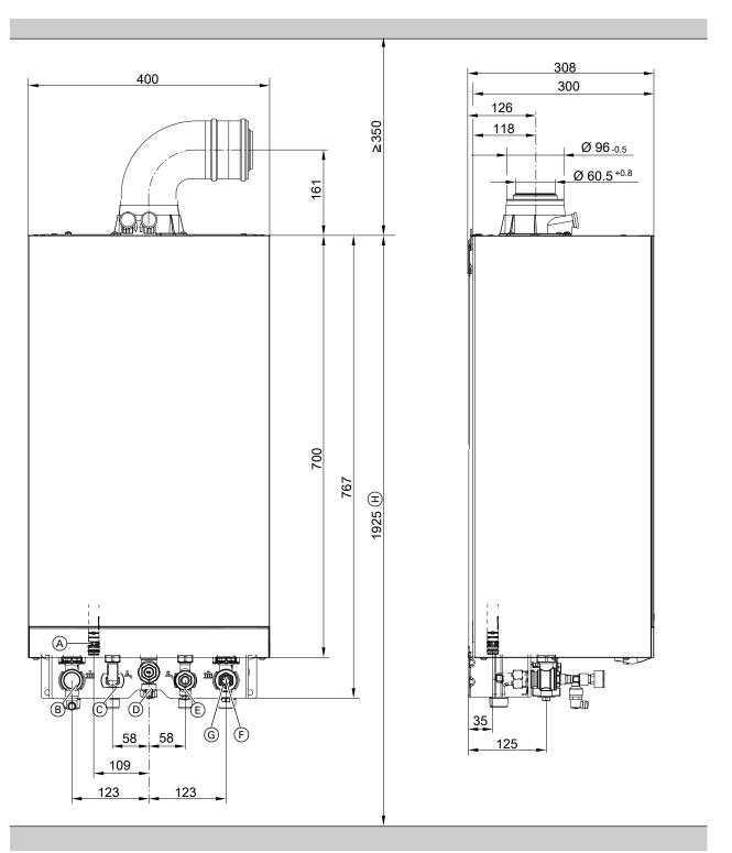
Fig. 2 Illustration shows a gas condensing combi boiler
