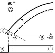
Fig. 47 Example 1: Changing the set room temperature from 20 to 26 °C
