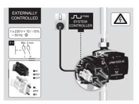
Fig. 65 Control box with Mini SS connection
