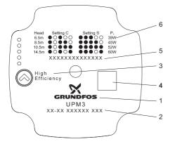
Fig. 6 Nameplate: Grundfos with setting indication
