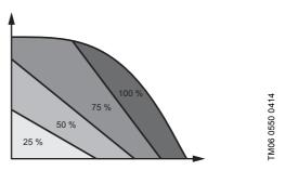
Fig. 22 Operation area according to performance load
