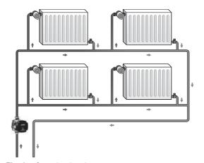
Fig. 2 One-pipe heating system
