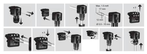
Fig. 67 Superseal installation plug
