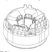
Fig. 38 Stator
