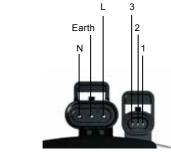
Fig. 63 Connections Mini SS
