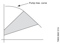
Fig. 30 Proportional pressure AUTO<sub>ADAPT</sub> operation area
