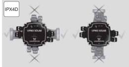
Fig. 53 Control box positions
