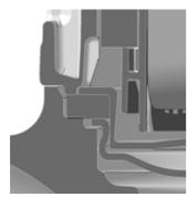
Fig. 48 Sectional drawing showing sealing principle of gasket
