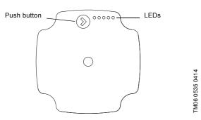
Fig. 21 User interface with one button and five LEDs
