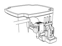
Fig. 70 FCI signal cable fixed by a separate lock
