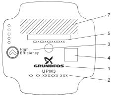
Fig. 7 Nameplate: customised layout
