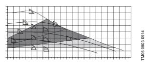
Fig. 25 UPM3 AUTO/HYBRID control modes with pump curves
