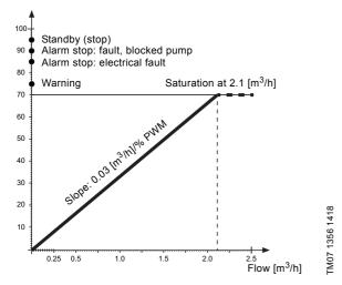
Fig. 18 PWM feedback signal - flow estimation
