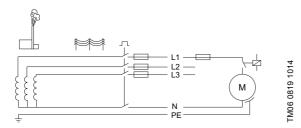
If you use a relay to switch the power supply of the pump, you risk excessive wear on the relay contact surface.
