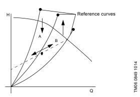
Fig. 33 Duty point on selected proportional pressure curve
