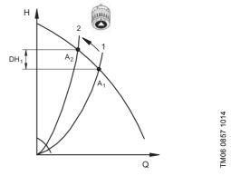
Fig. 27 Uncontrolled pump
