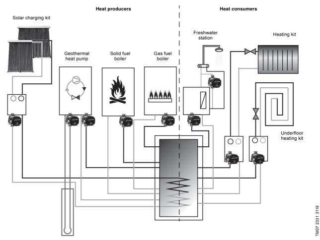
Fig. 1 Complete domestic heating system combined with renewable energy sources
