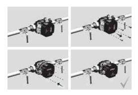
Fig. 54 Changing the control box position
