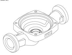
Fig. 49 Pump housing
