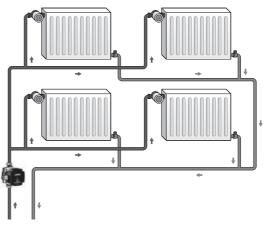
Fig. 3 Two-pipe heating system
