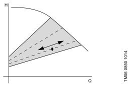
Fig. 34 New lower proportional pressure curve
