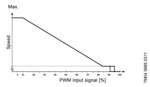
Fig. 14 PWM input profile A (heating)
