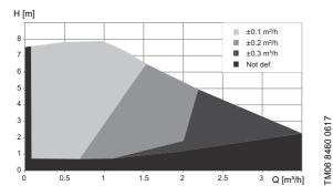
Fig. 19 Accuracy of PWM feedback signal - flow estimation with water at 20 °C
