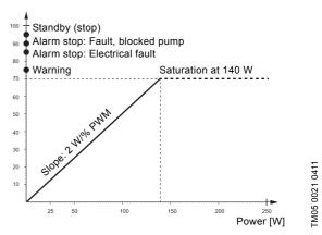
Fig. 17 PWM feedback signal, UPM3L power consumption
