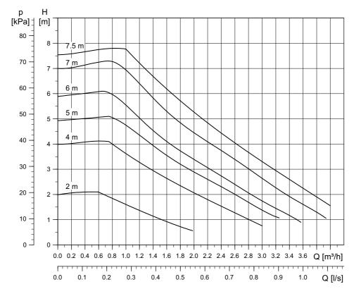
Fig. 9 Performance range UPM3, cast iron pump housing
