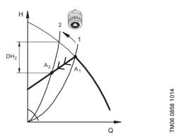
Fig. 28 Pump operated in proportional-pressure control mode
