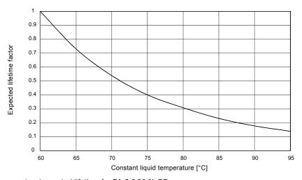
Fig. 51 Diagram temperature/expected lifetime for PA 6.6 30 % GF
