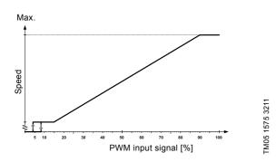
Fig. 15 PWM input profile C (solar)
