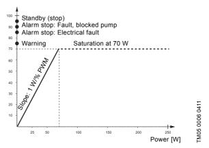
Fig. 16 PWM feedback signal, UPM3 power consumption
