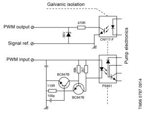
Fig. 13 Schematic drawing, interface
