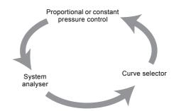
Fig. 29 The AUTO<sub>ADAPT</sub> three-step task
