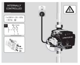
Fig. 64 Control box without signal connection
